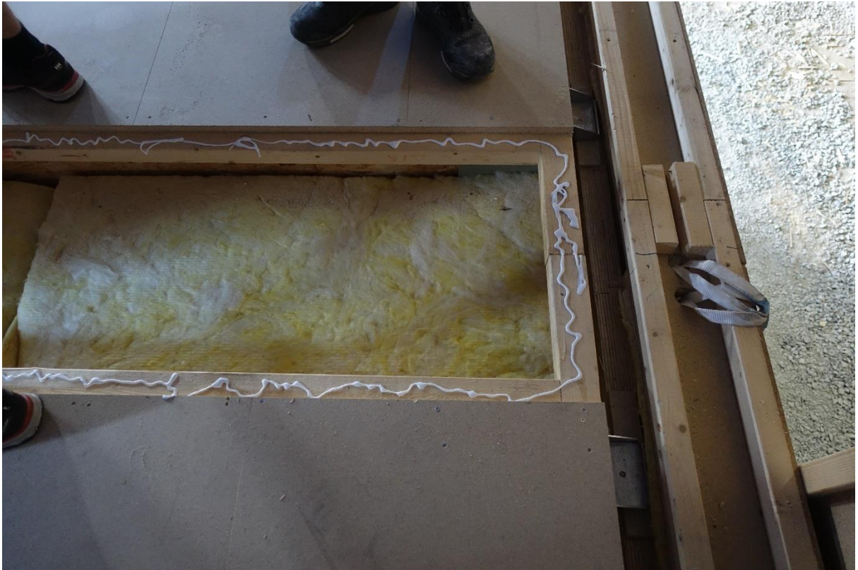
Figure 9. Test setup version 3, gluing and screwing of the particleboards to the joist in the floor.
