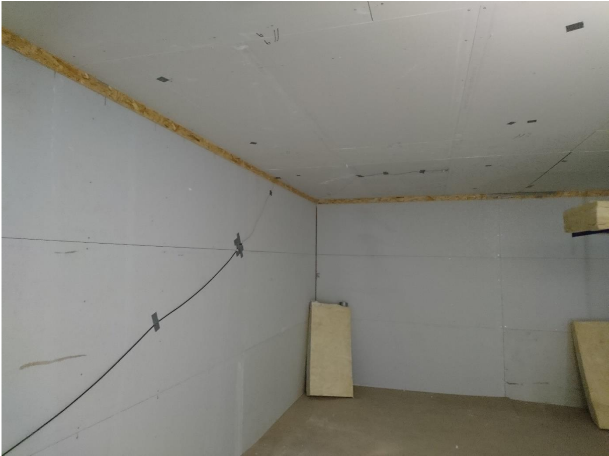
Figure 13. Test setup version 8, OSB strips fastened in the corners to represent the use of cornices.
