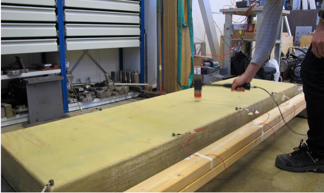
Figure 2.2- Performing natural frequency measurements
