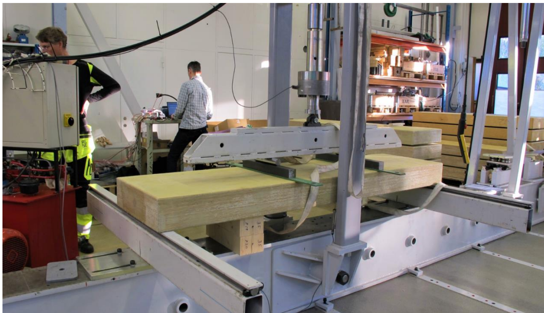
Figure 2.1- Performing the four-point bending test.
