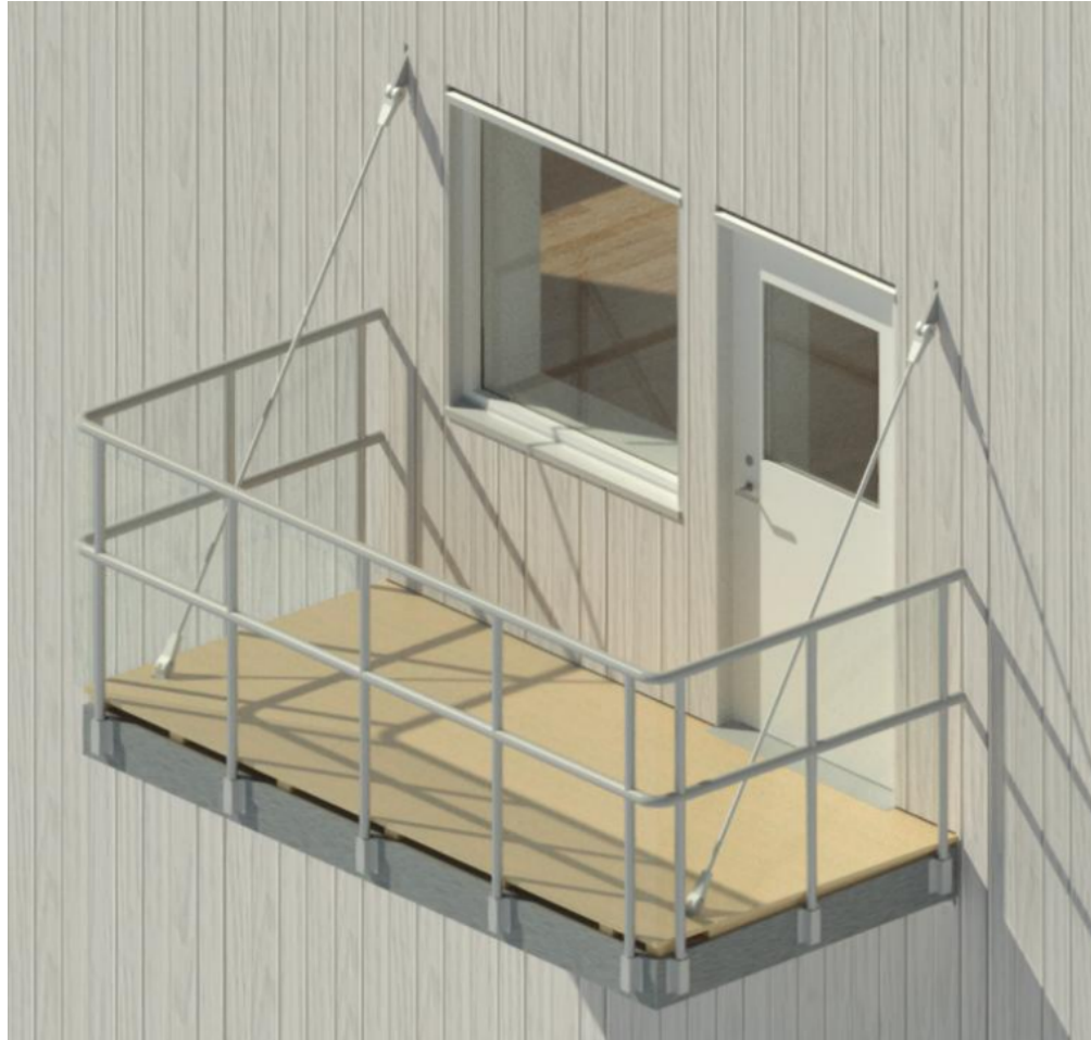
(a) Rendered picture of the real balcony. The wall-side is fixed by steel brackets, the other two sides are supported by steel rods [1] .
