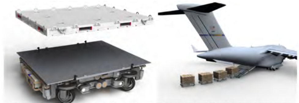
(Left) Holonomic mobile platform with high strength actuators; (Right) The wireless i -Pbot swarms navigate autonomously at the proper location on the aircraft with weight distribution.
